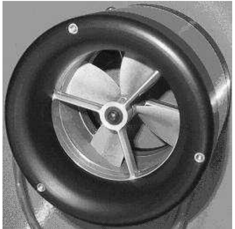
Fig. 1: Photograph of a commercial rim-driven thruster designed by the Authors
