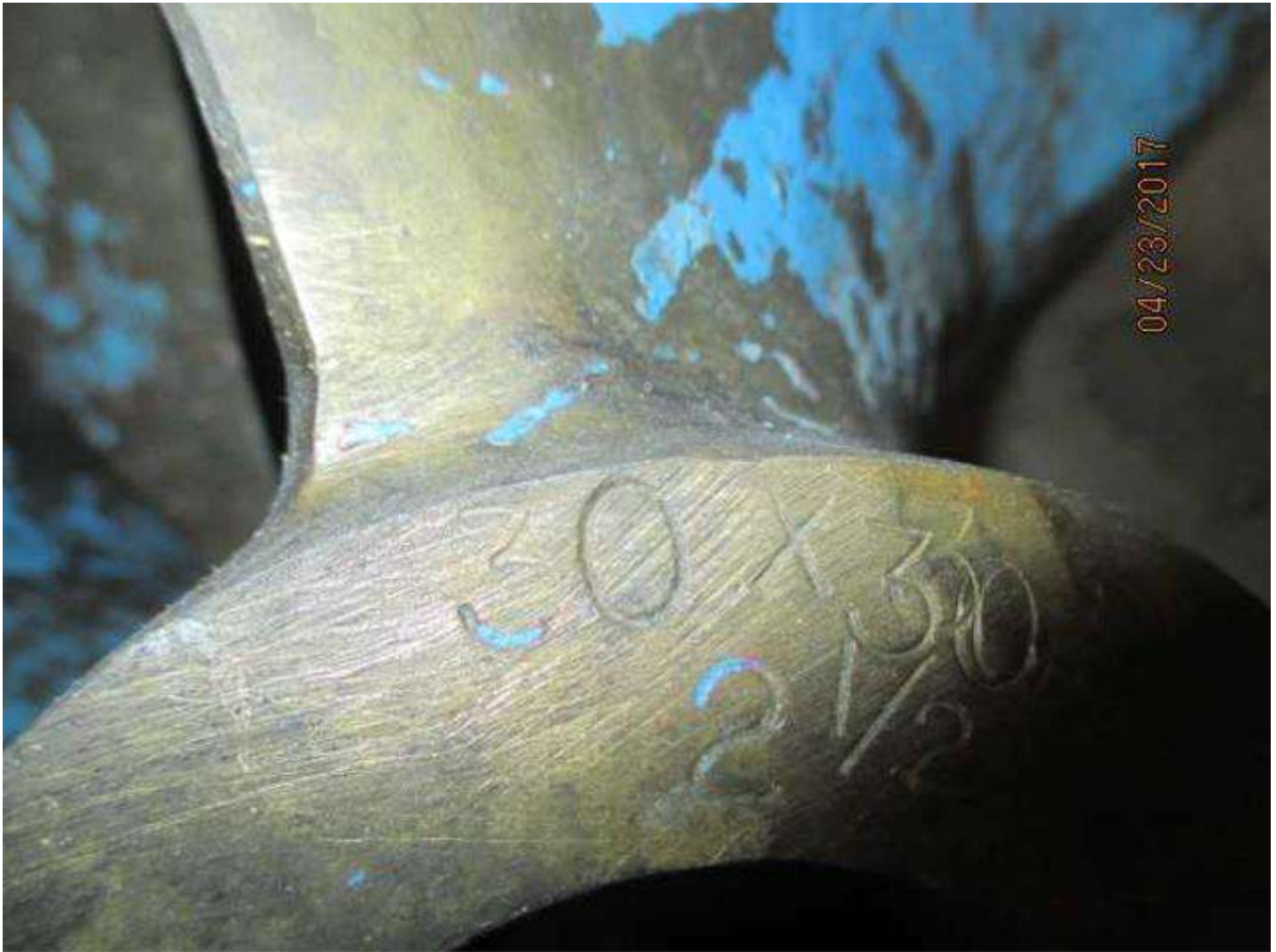
265 280-IMG_0007 Date Taken: 4/23/2017 Taken By: Ray Bilbrey ONE SET RIGHT AND LEFT HAND 4 BLADE 30"X30"X2 1/2" BRONZE PROPELLERS FOR MOTOR YACHT
